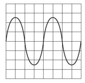
Each horizontal division on the oscilloscope screen represents 0.002 s.
