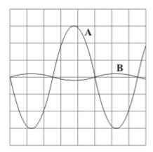
Trace  $\bf A$  shows how the potential difference between the live and neutral terminals of an electricity supply changes with time.
